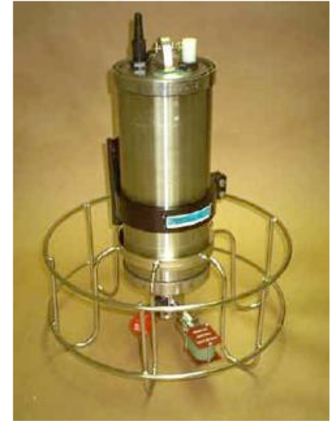
CTD (conductivity, temperature, pressure) for measuring conductivity in a profile (on the fly)
